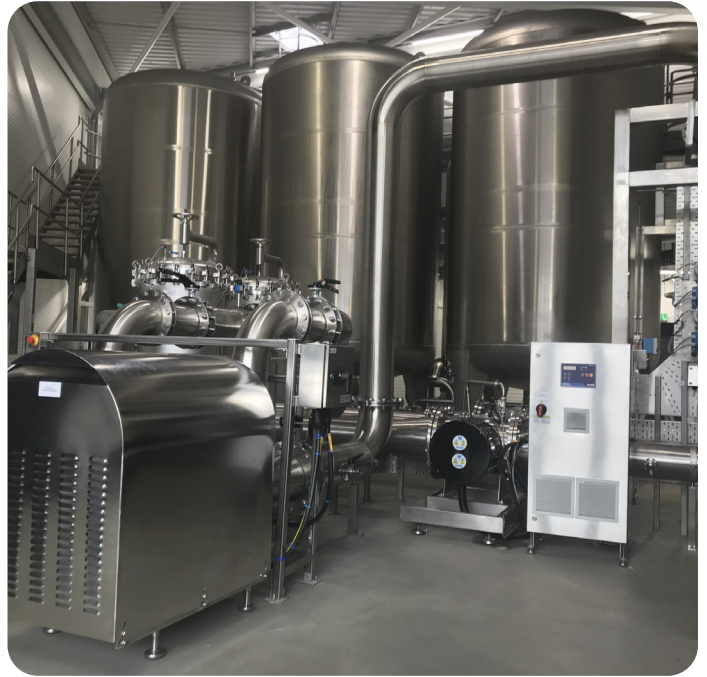
The finished build on-site, showing the stainless steel vessels and feed pump system.
