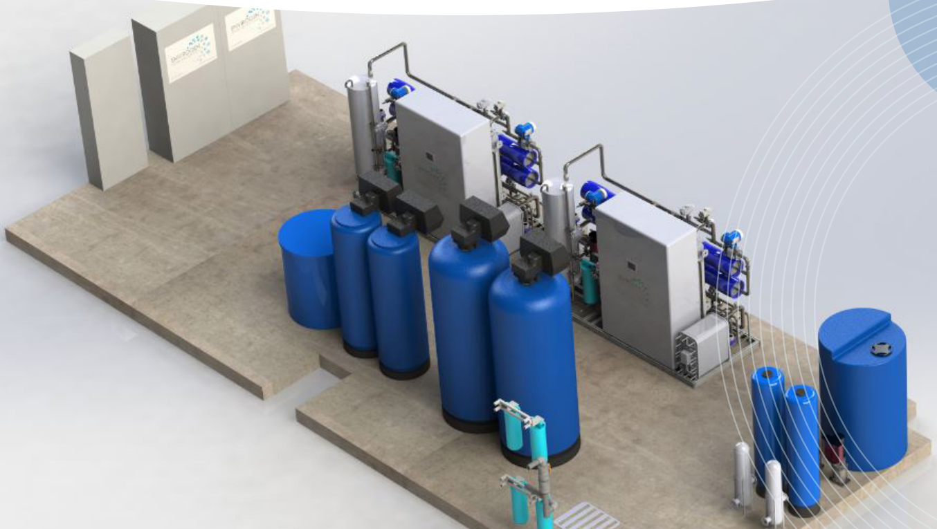
3D model designed to show the final demin water plant installed at Energy Works Hull
