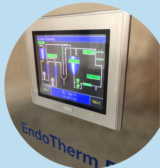
Highly resilient reverse osmosis plants from Envirogen: Two duplex EndoTherm Duo RO units shown with full colour touchscreen HMI monitors
