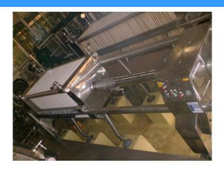
hydraulic seal kit. All seals replaced – plate, frame, profile and end plate seals and carried out a seal service to prevent future breakdown.
