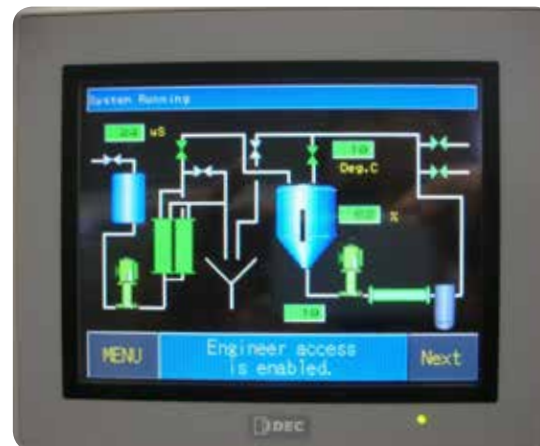
PLC controller with colour touch screen HMI for easy system programming
