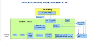
**Project:** Containerised system delivering European Pharmacopia / USOP grade water for use as an ingredient in the production of prescription tablets.
