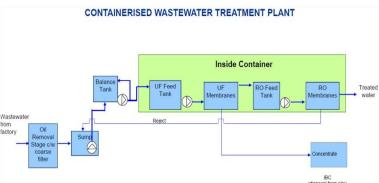
**Project** - Conatinerisd plant reducing pollutants within trade wastewater. To remain in compliance for discharge to sewere and have the potential to reuse treated water.
