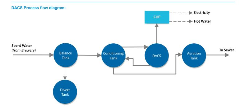
Mark Little explains how it works: "The wastewater is screened and held in a balance tank, where the flow and concentration of the wastewater is continually mixed to form a homogenous feed to the next process stage. The wastewater is then directed to the conditioning tank where it is mixed with some of the anaerobically treated wastewater."
